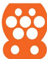
CCS - 50kW DC
